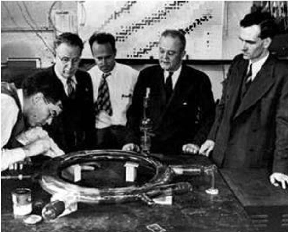
**Fig. 1.** General Electric Scientists inspecting the vacuum chamber of the 70-MeV synchrotron in which synchrotron radiation was first observed. *Left to right:* Robert Langmuir, Frank Elder, Toly Gurewitsch, Ernest Charlton, and Herb Pollock.
