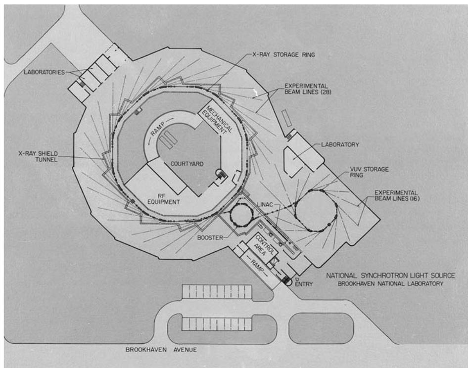
**Fig. 8.** The NSLS design in the proposal of February 1977, showing the large X-ray storage ring in the upper left and the Vacuum Ultraviolet (VUV) storage ring in the lower right. *Credit:* Brookhaven National Laboratory.
