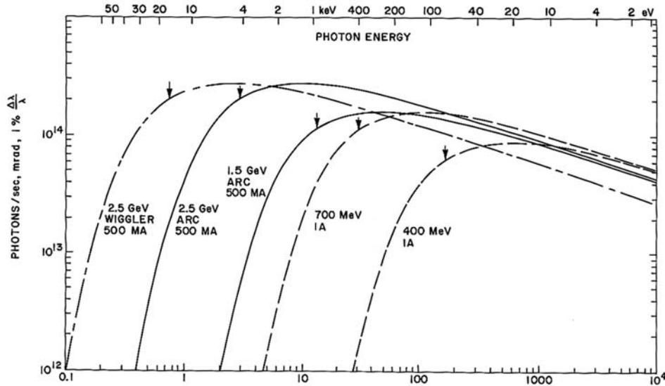
**Fig. 4.** The light given off by a synchrotron-radiation source. The wavelength of the light is plotted against the number of photons emitted per second. As the wavelength decreases (or the frequency or photon energy increases), the number of photons emitted per second (or photon intensity) increases slowly and then abruptly falls to zero. *Credit:* Brookhaven National Laboratory.
